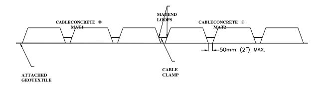
WHENPLACING THE MATS, THE GAPBET WEEN THE MATSSHOULD NOT BEANYLARGER THAN A 50 mm (2'') MAXIMUM. IF THE MATS A REPLACED WITH A LARGER SPACE THAN 50 mm (2''), IT IS RECOMMENDED TO GROUT THESE AMBET WEEN THE MATS.
