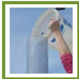
Figure 9: Filling Infiltrometer with Water
