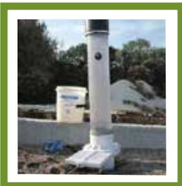
Figure 7: Infiltrometer Placement
