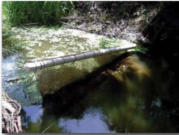
Figure 29. Particle curtain in a canal
