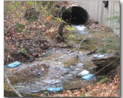
Figure 25. Six of the polymer blocks placed downstream
