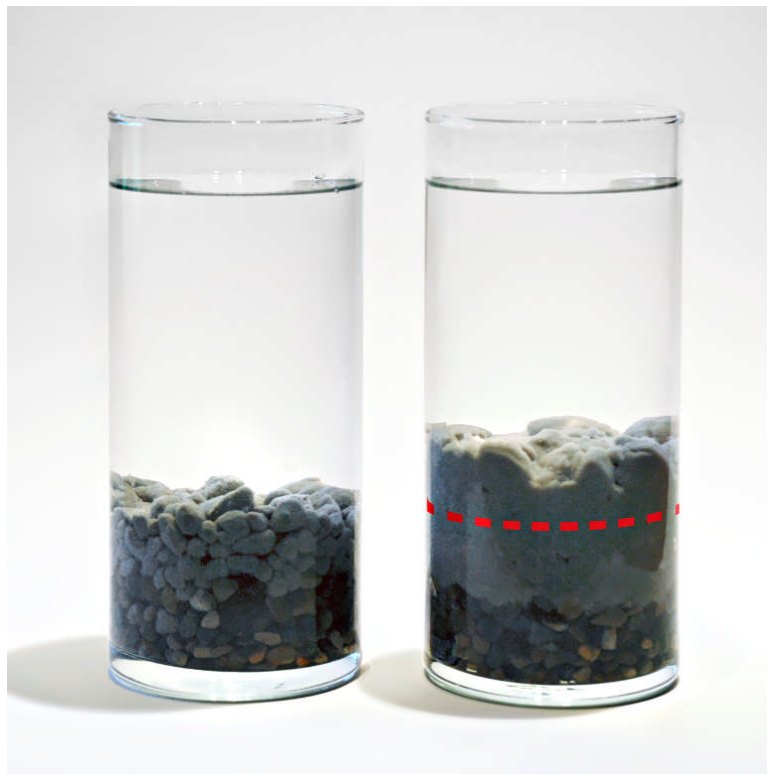
Figure 1. PONDSEAL™ applied at 7-lbs./ft 2 five minutes after inundation (left) and 24 hours after inundation (right). Note original boundary between product and water (dashed red line) demonstrating swell/expansion of product over time.
