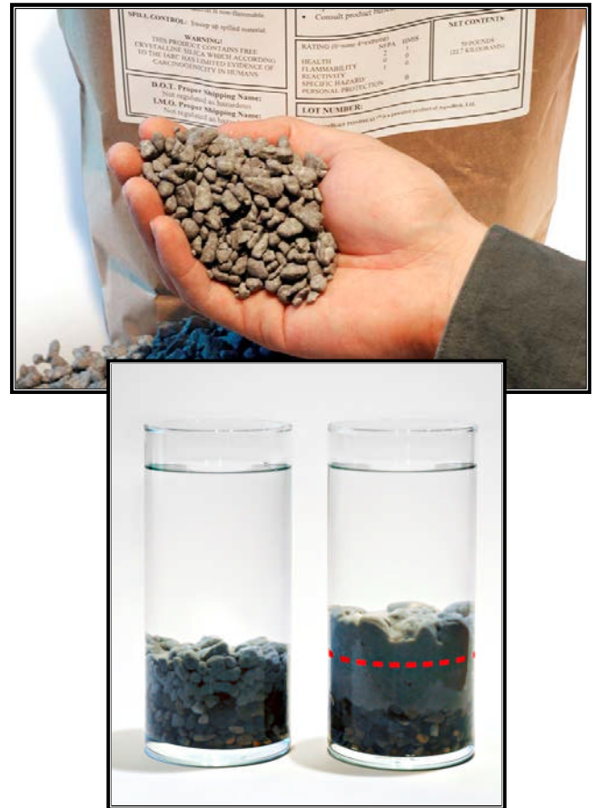
Figure 1. Configuration of stone-clay composite particle.
