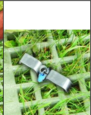
Figure 9. Loop cable back in the Gripple
