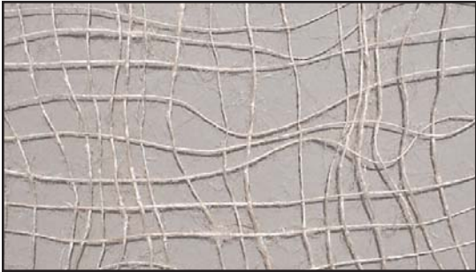
Leno woven nets (above) feature double twisted strands in the machine direction that provide higher strength and integrity to the BioNet blankets than that of cross-lay nets (below).
